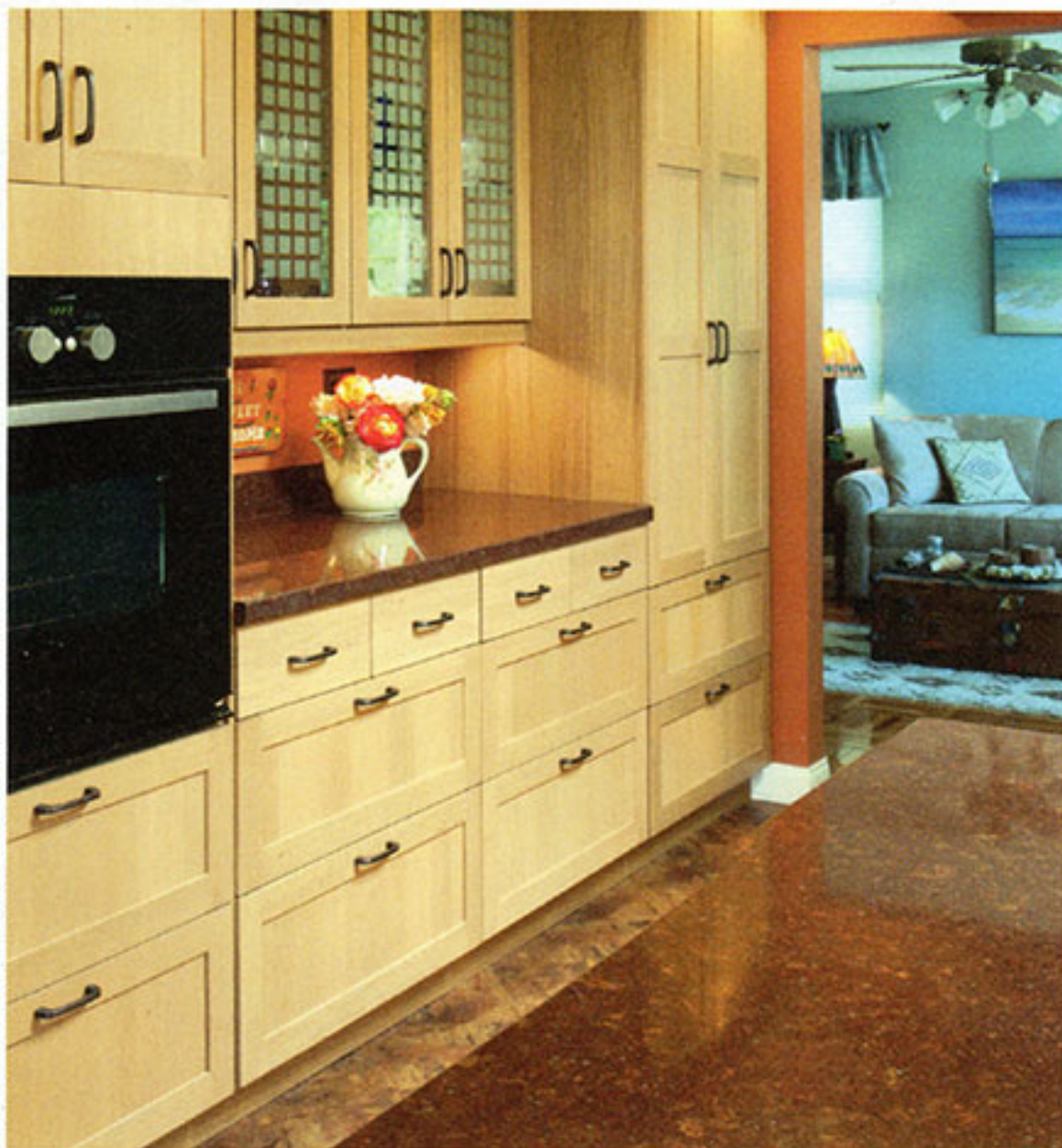
The remodeling of this kitchen involved lowering the oven, installing easy-grasp handles and pull-out shelves behind pantry doors, widening the doorway into the living room and adding lighting, including under the cabinets.
